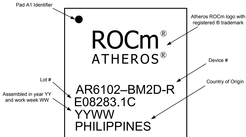
Figure 7-1. AR6102 Package Marking
