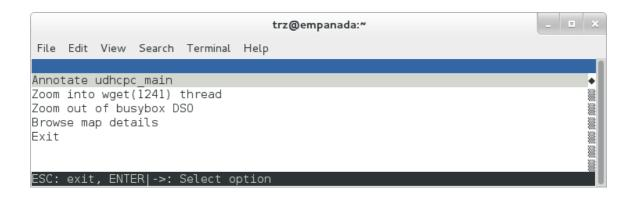
Selecting 'Annotate udhcpc\_main', we get a detailed listing of percentages by instruction for the udhcpc\_main function. From the display, we can see that over 50% of the time spent in this function is taken up by a couple tests and the move of a constant (1) to a register:
