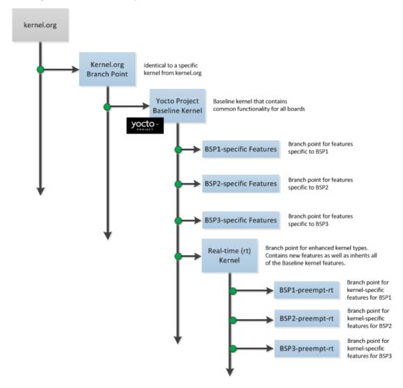
In the illustration, the "Kernel.org Branch Point" marks the specific spot (or Linux kernel release) from which the Yocto Linux kernel is created. From this point forward in the tree, features and differences are organized and tagged.
