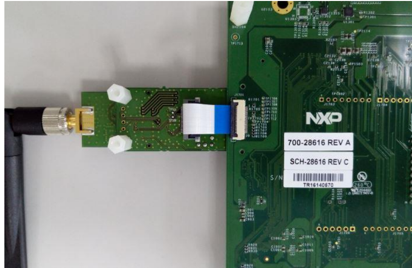
Figure 11. Connect the BT module
