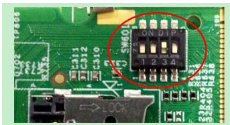
Figure 5. SW601 boot device settings
