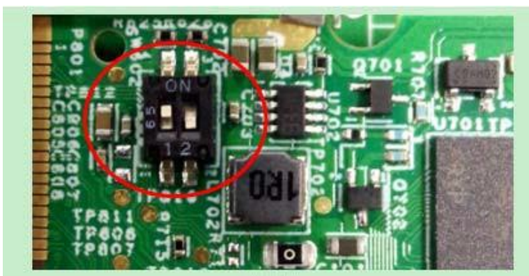
Figure 4. SW602 boot mode settings
